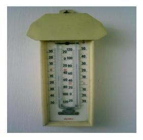
Figure 2: A Typical Outdoor Minima-Maxima Thermometer
