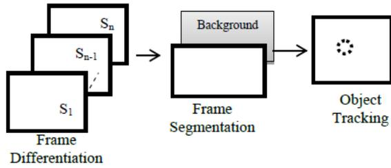
Figure 2.1: Basic Block- Object Video Tracking (Prakash & Shalini, 2011)
