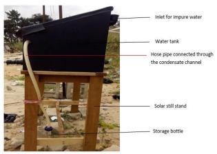
**Fig. 2.** Side view of the slanting-type solar water distillation (SSWD) kit
