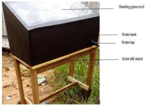
Fig. 1. Front view of the slanting-type solar water distillation (SSWD) kit
