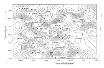
FIG.4 CONTOU MAP OF AQUIFER THICKNESS (CONTOU THICKNESS 2m)
