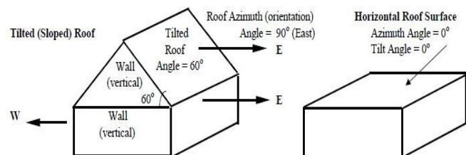
**Figure 2:** Orientation (Azimuth) and direction (<http://energy-models.com/azimuth-angles-building-surfaces>).
