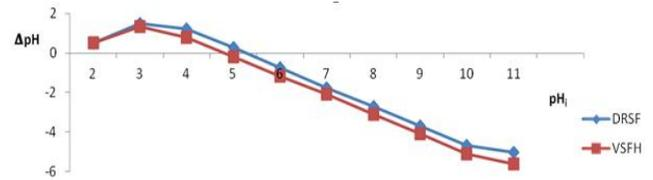
Fig. 2: Plots of  $\Delta\text{pH}$  against  $\text{pH}$  showing points of zero charge of DRSF and VSFH
