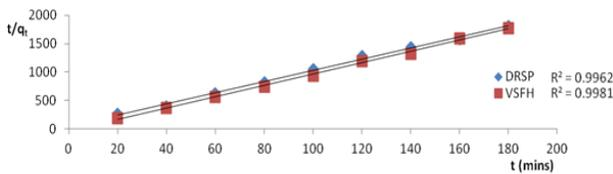
Fig. 8: Pseudo-second order plot for methylene blue adsorption on DRSP and VSFH
