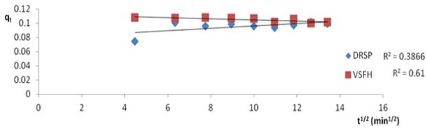
Fig. 6: Intraparticle diffusion plot for methylene blue adsorption on DRSP and VSFH
