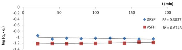
Fig 7: Pseudo-first order plot for methylene blue adsorption on DRSP and VSFH
