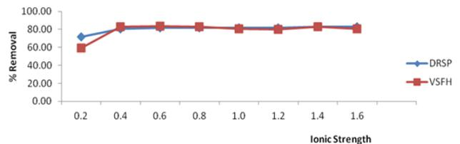
Fig. 4: Plots of removal efficiency against ionic strength
