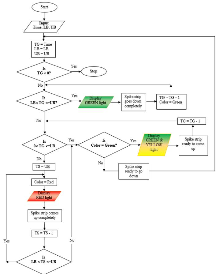
Figure 1: Flowchart Diagram for Traffic Light System using Smart Spike Strip (SSS) for one lane at the traffic Junction
