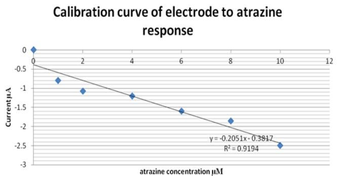
**Figure 5:** Calibration curve of successive additions of atrazine responses at modified electrode in 0.32 mM of atrazine solution at pH 5 at scan rate of 50 mV/s
