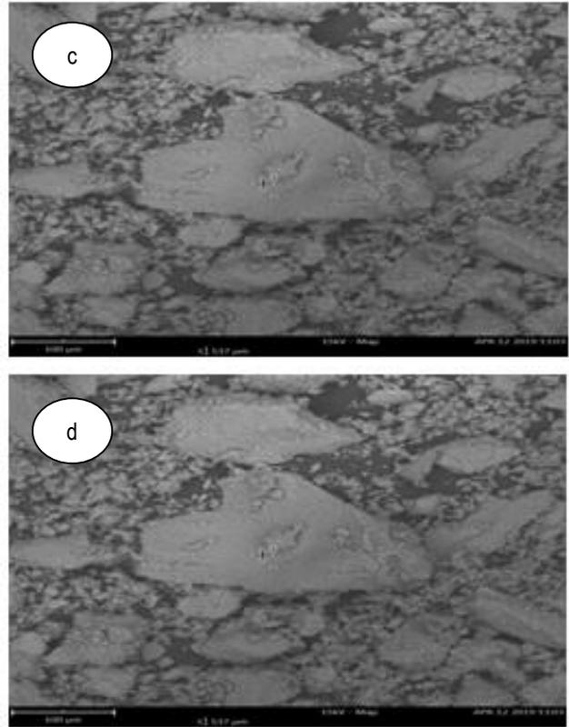
**Plate:** SEM morphology of (a) Bare Graphite Electrode (b) Graphite with Emeraldine (c) Graphite with Hkust-1 and (d) Graphite with Emeraldine and Hkust-1
