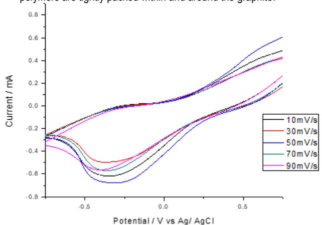
**Figure 1:** Cyclic Voltammogram showing the effect of scan rate of 10-90 mV/s in 0.32 mM atrazine solution at (pH 3) supporting electrolyte.
