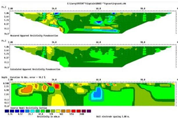
**Figure 8:** 2D inversion result of profile 6. (a) measured apparent resistivity pseudo-section, (b) calculated apparent resistivity pseudo-section, and (c) inverse model resistivity section.
