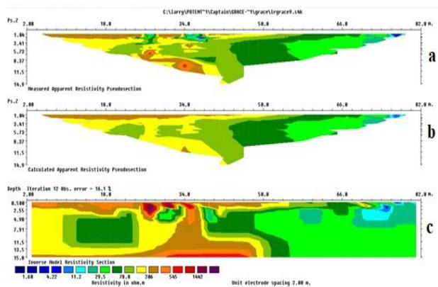
**Figure 12:** 2D inversion result of profile 10. (a) measured apparent resistivity pseudo-section, (b) calculated apparent resistivity pseudo-section, and (c) inverse model resistivity section.
