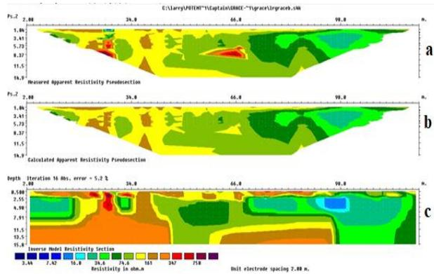
**Figure 11:** 2D inversion result of profile 9. (a) measured apparent resistivity pseudo-section, (b) calculated apparent resistivity pseudo-section, and (c) inverse model resistivity section.
