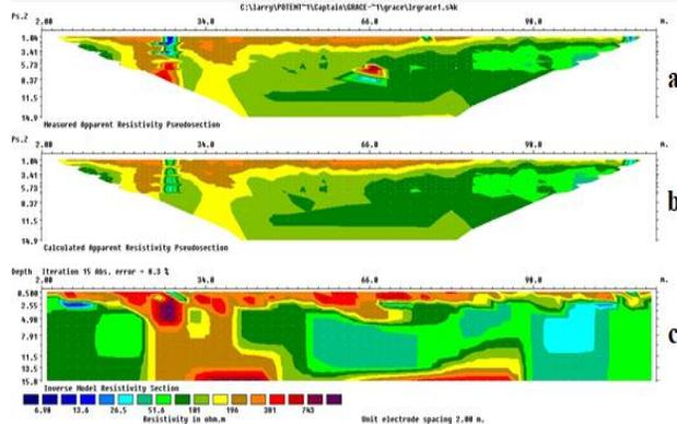
**Figure 3:** 2D inversion result of profile 1: (a) measured apparent resistivity pseudo-section; (b) calculated apparent resistivity pseudo-section; and (c) inverse model resistivity section.
