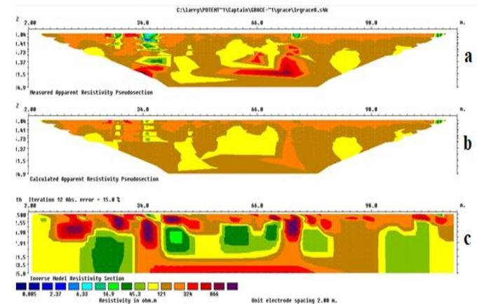
**Figure 10:** 2D inversion result of profile 8. (a) measured apparent resistivity pseudo-section, (b) calculated apparent resistivity pseudo-section, and (c) inverse model resistivity section.
