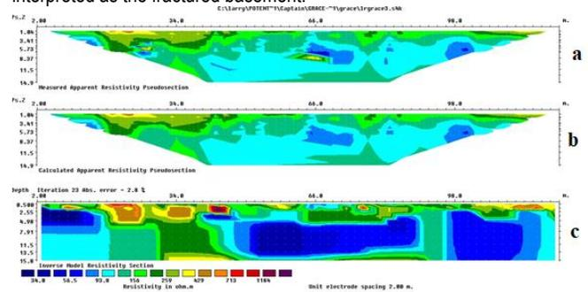
**Figure 5:** 2D inversion result of profile 3. (a) measured apparent resistivity pseudo-section, (b) calculated apparent resistivity pseudo-section, and (c) inverse model resistivity section.
