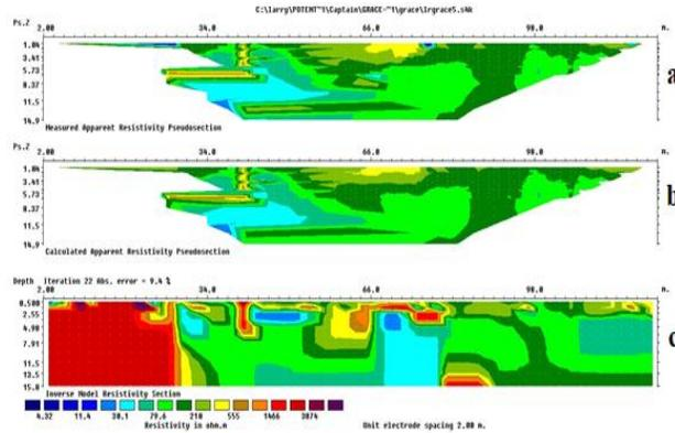
**Figure 7:** 2D inversion result of profile 5. (a) measured apparent resistivity pseudo-section, (b) calculated apparent resistivity pseudo-section, and (c) inverse model resistivity section.
