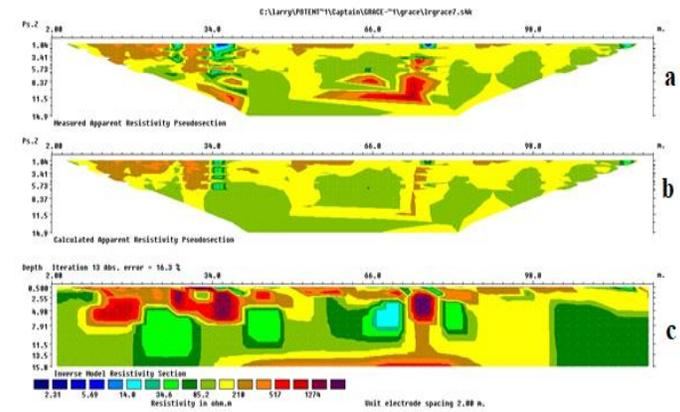
**Figure 9:** 2D inversion result of profile 7. (a) measured apparent resistivity pseudo-section, (b) calculated apparent resistivity pseudo-section, and (c) inverse model resistivity section.
