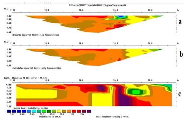
**Figure 13:** 2D inversion result of profile 11. (a) measured apparent resistivity pseudo-section, (b) calculated apparent resistivity pseudo-section, and (c) inverse model resistivity section.
