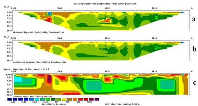
**Figure 4:** 2D inversion result of profile 2. (a) measured apparent resistivity pseudo-section, (b) calculated apparent resistivity pseudo-section, and (c) inverse model resistivity section.
