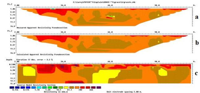
**Figure 6:** 2D inversion result of profile 4. (a) measured apparent resistivity pseudo-section, (b) calculated apparent resistivity pseudo-section, and (c) inverse model resistivity section.
