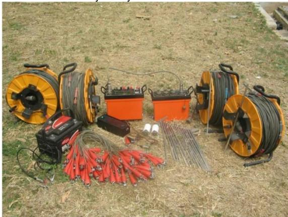
**Figure 2:** The ABEM LUND imaging system and the Terrameter SAS1000
