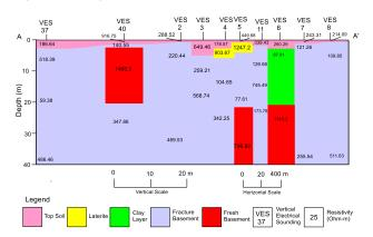
Figure 6: Geoelectric section of profile B-B
