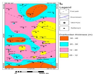
Figure 4: showing overburden thickness
