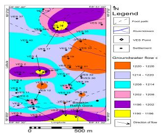
Figure 10: Groundwater flow direction
