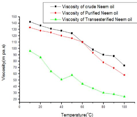
Figure 2: graph of viscosity against Temperature
