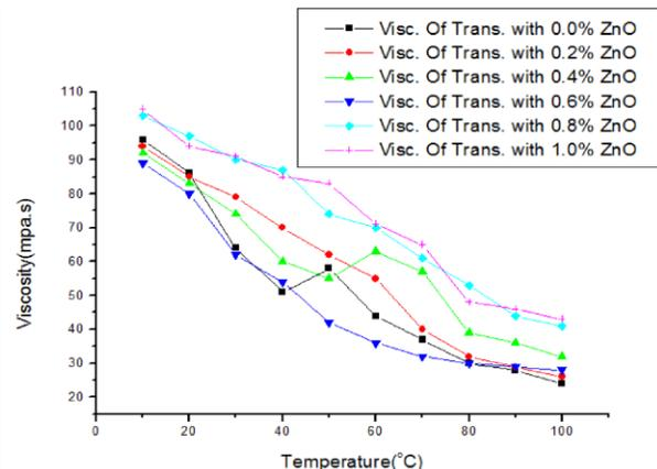
Figure 3: Graph of Viscosity of Nano fluid against Temperature
