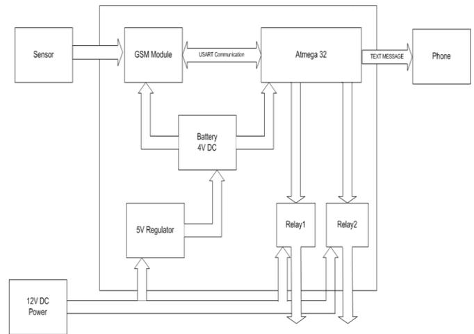
Figure 2: Hardware block diagram
