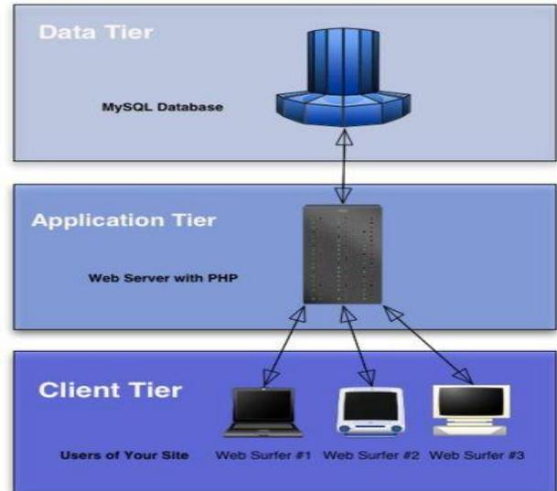
Figure 5: System architecture
