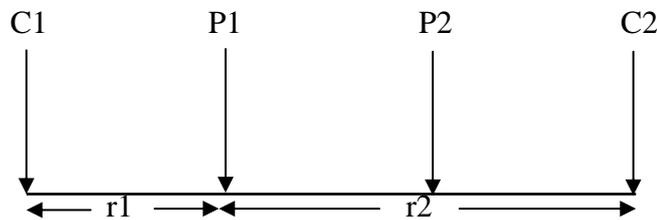
FIG. 3 ELECTRODES CONFIGURATION
