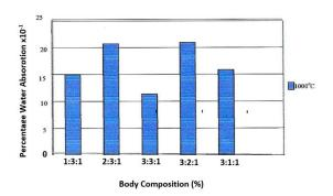
Figure 2: Water Absorption at 1000°C
