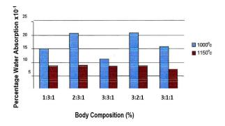
Figure 3: Chart showing Water Absorption at 1000°C and 1150°C
