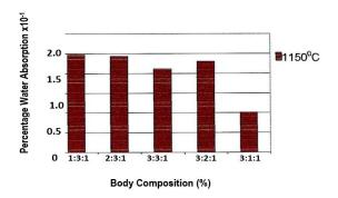
Figure 1: Water Absorption at 1150°c
