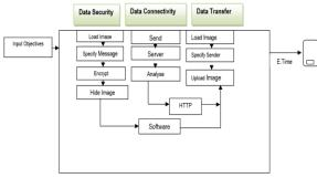
Fig 2: The System Architecture
