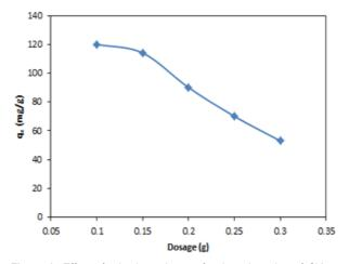
Figure 2: Effect of adsorbent dosage for the adsorption of CV onto cornstalk
