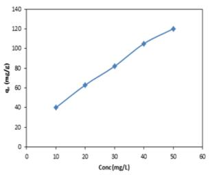
Figure 3: Effect of changing dye Concentration for the adsorption of CV onto Cornstalk.
