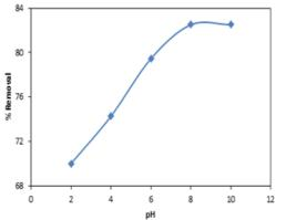
Figure 4: Effect of pH for the adsorption of CV onto corn stalk.
