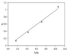
Figure 5: Langmuir isotherm model for the adsorption of CV on CS
