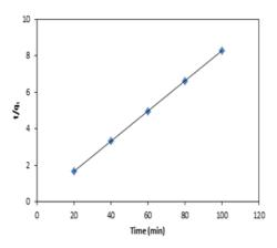
Figure 8: Pseudo-second order kinetic model for the adsorption of CV onto CS
