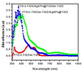
Fig. 3c. UV-vis spectra of various prepared Photoanodes after dye sensitization
