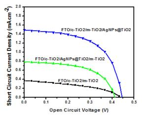
**Fig. 4.** Photocurrent density-voltage (*J-V*) curve under 100 mWcm<sup>-2</sup> light intensity
