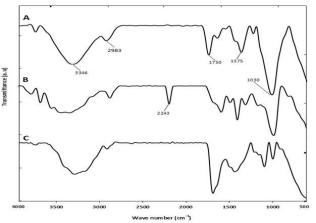
**Figure 1:** FT-IR spectra of (a) PSP (CS) (b) poly(AN-*g*-PSP) & (C) amidoxime- modified poly(AN-*g*-PSP)
