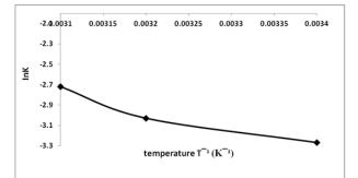
**Figure 6:** Temperature effect on the adsorption of methylene blue onto amidoxime-modified poly(AN-*g*-PSP) (Volume of the MB dye solution: 50 ml, Adsorbent dosage: 0.3g, Temperature: 298 K, 308 K, 318 K, Initial concentration of MB 100 ppm, pH: 6.5, Particle size: 75-300
