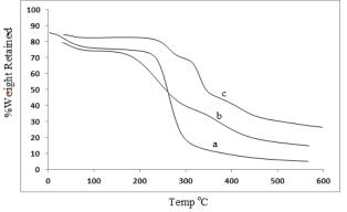
**Figure 2:** TG and DTG curves of (A) PSP (B) poly(AN-*g*-PSP) and (C) amidoxime-modified poly(AN-*g*-PSP).
