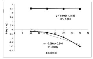
Figure 4: The Pseudo first-order kinetics plot for the sorption of methylene blue dye onto amidoxime-modified poly(AN-g-PSP).
