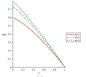
Figure 1: Graph of velocity u(y) against distance, y for different values of power law index when  $\delta = 0.5, \gamma = 1, D_0 = 1, \alpha = 0.2, K_0 = 0.4, \varepsilon = 0.01, n = 0$ ,  $\beta = 0.5$
