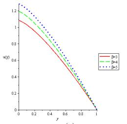
**Figure 2.:** Graph of velocity u(y) against distance y for different gradient coefficient  $\beta$  when values of pressure  $\delta = 0.5, \gamma = 1, D_0 = 1, \alpha = 0.2, K_0 = 0.4, \varepsilon = 0.01, n =$  (different values of Frank Kamenetskii number  $\delta$  when ,m=1
