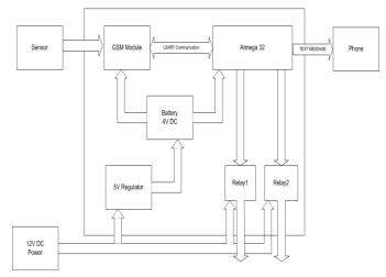
Figure 2: Hardware block diagram
