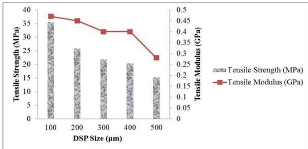
**Figure 2:** Effect of Particle Size on Tensile Strength and Modulus of DSP-UPR Composites
