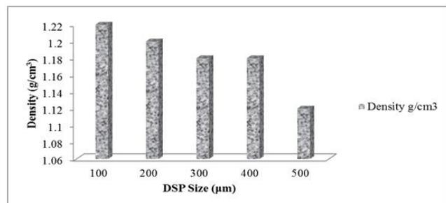
**Figure 4:** Effects of Particle Size on Densities of UPR-DSP Composites
